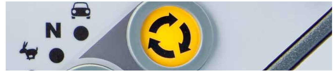
3 Conveyor movement reversible for a short time
